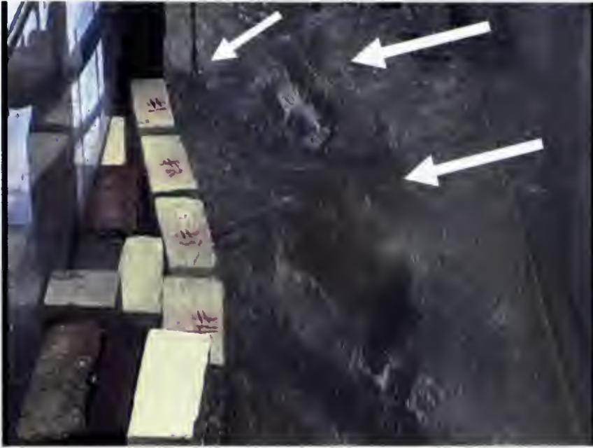
**Figure 6.10** Clip 1 of a sequence of photos taken for an experimental run. The initial depth of the flume is 5.8cm and there was no offset. This is the initial position of the blocks, which are marked with red numbers, before block #1 (top of photo) began to move. Larger arrows are highlighting the crests of standing waves. Smaller arrow is highlighting the location of the ADV. Flow is moving from the top of the photo to the bottom.
