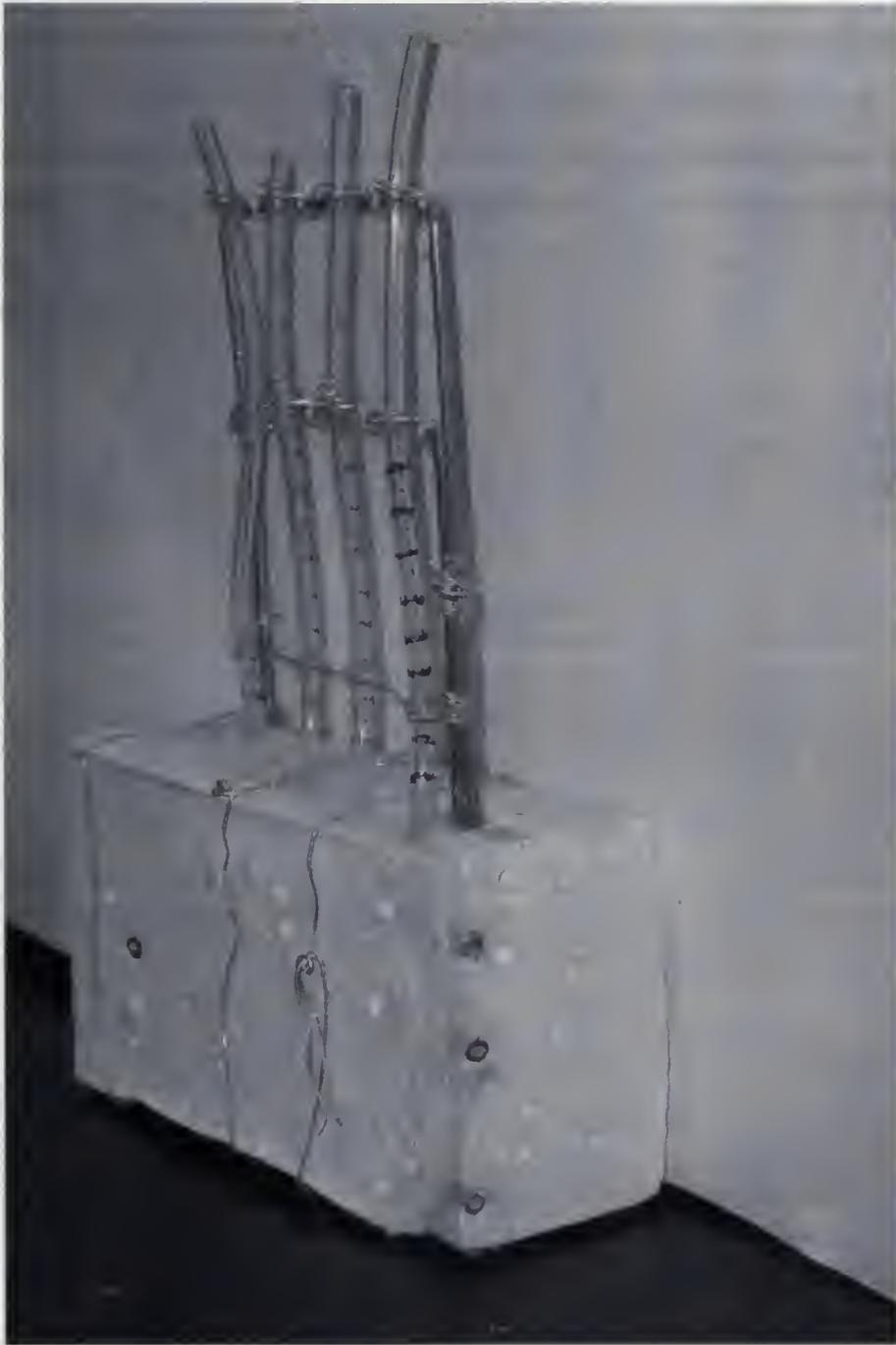
**Figure 5.6** Picture of the constructed tube block used to collect velocity data by measuring the water height in the tubes and using the velocity head formula.
